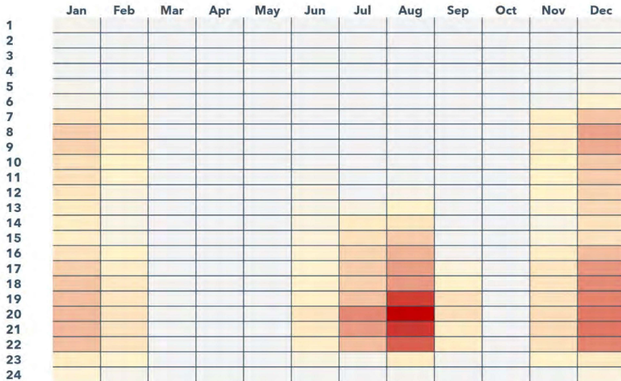
Figure 3: Capacity Need Heatmap, Figure 44 from PGE's 2023 IRP
