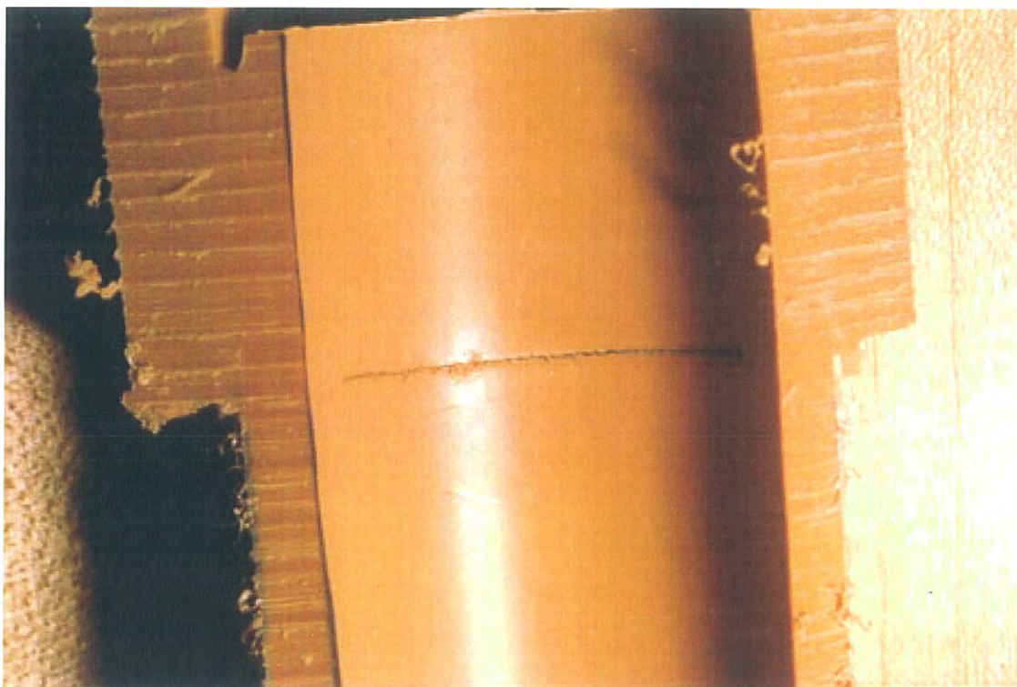
Figure 7 -- Interior of polyethylene pipe from San Juan pipeline accident showing brittle-like crack with no visible deformation.
