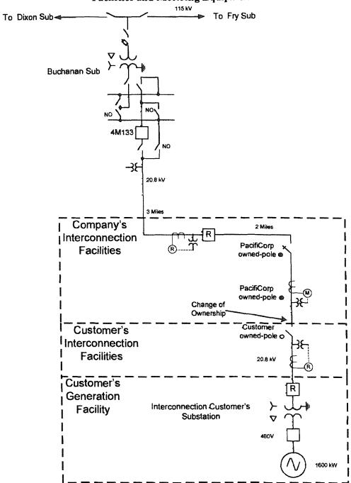
One-line Diagram Depicting the Generating Facility, Interconnection Facilities and Metering Equipment
