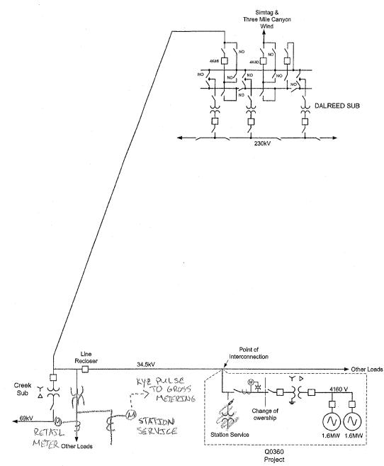
Figure 1: System One Line Diagram
