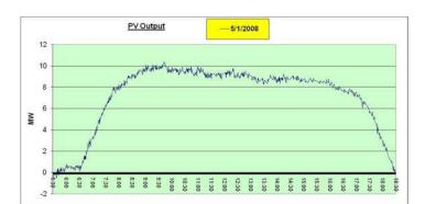
Figure 2. Solar Photovoltaic Plant Output on a Sunny Day at a Nevada Site $^{216}$
