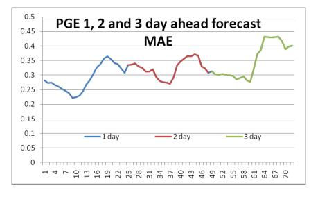
Figure 3: Mean Absolute Error for PGE wind forecasts of 1, 2, and 3 days ahead
