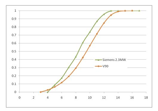
Figure 2: V90 and Siemens 2.3 MW power curves
