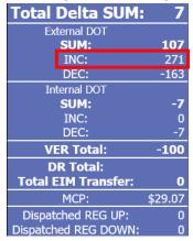
DEC: Sums up the RTD/RTPD External DOT DEC, VER DOT DEC, and DR DOT DEC numbers shown on the Dispatch Control Screen and compares that to the Actual Generation DEC Threshold.
