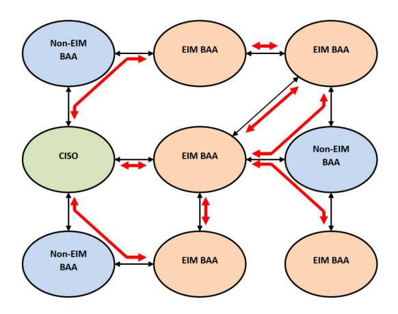
EIM BAAs may be interconnected with the CISO directly, through another WEIM BAA, through a Non-EIM BAA, or a combination thereof. The WEIM Entity for an WEIM BAA may have made available transmission rights on a direct interconnection with the CISO, on a direct interconnection with another WEIM BAA, or on an indirect interconnection with the CISO or another WEIM BAA through one or more
