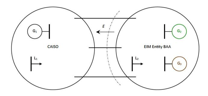
The power transfer (E) between the BAAs is limited to 100MW. The resource data is as follows:
