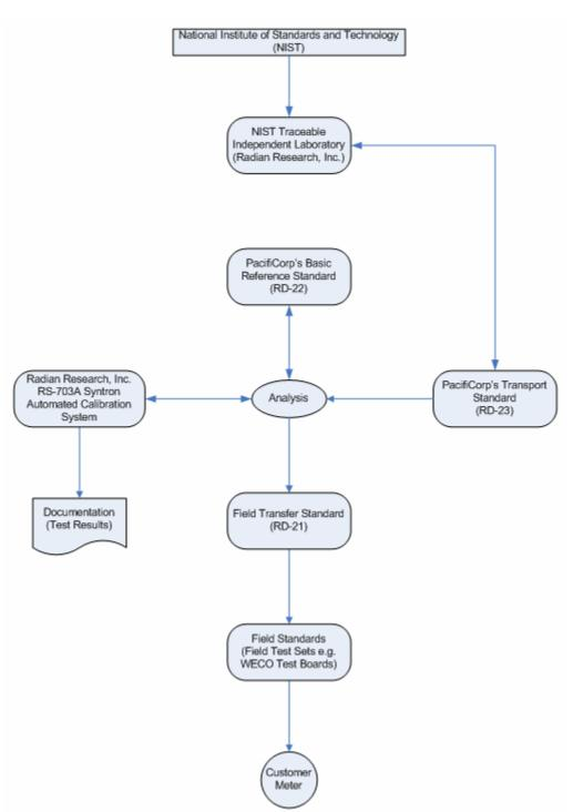
Figure 1 - PacifiCorp's traceability diagram
