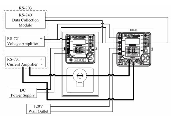
Figure 1 – Equipment setup for quarterly certification
