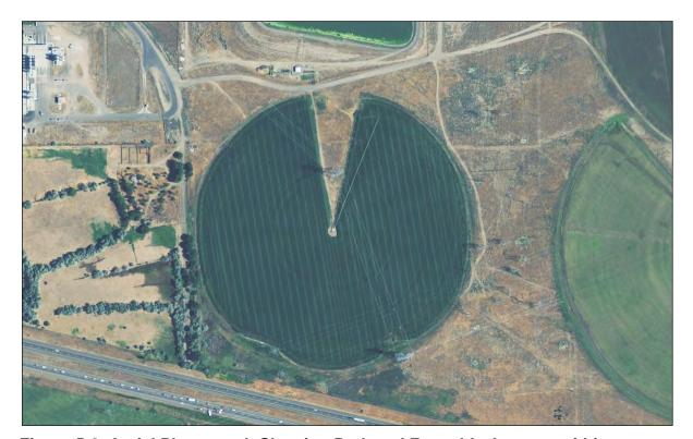
Figure 5-2. Aerial Photograph Showing Reduced Farmable Acreage within a Center-Pivot-Irrigated Parcel Resulting from the Placement of a Transmission Line Tower (approximately 2 acres of this 40-acre field are lost to production because of the presence of a transmission line tower)
