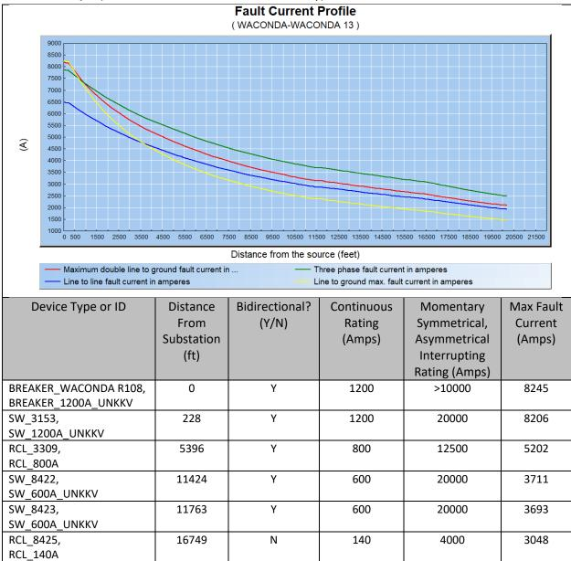
**Note:** List devices between proposed point of interconnection and the feeder breaker. Include feeder regulator(s), feeder breaker, fuses, reclosers, switches, sectionalizers, and line regulators
