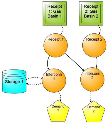
In this simple diagram there are two supply basins, two demand areas, and a single storage facility. There are pipelines that connect Gas Basin 1 to both demand areas, but gas from Gas Basin 2 can only flow to demand area 2. There are two dashed arrows between Storage 1 and Interconnect 1; indicating that gas from Interconnection 1 can flow both in an out of the storage facility.
