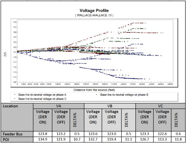
**System Backfeed** (Record loading at the source side of the proposed DER facilities' feeder breaker, and at the distribution power transformer).
