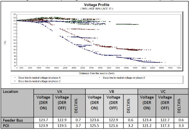
**System Backfeed** (Record loading at the source side of the proposed DER facilities' feeder breaker, and at the distribution power transformer).
