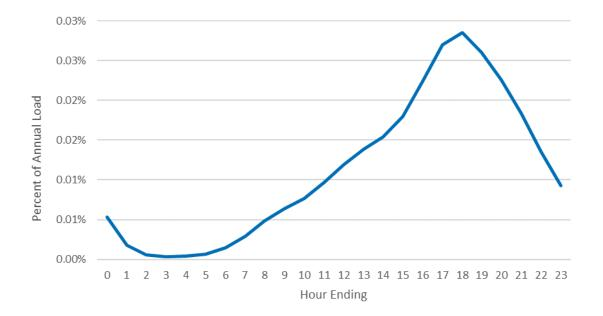
This load shape shows EV load peaking at hour 18 or 6:00 pm, which coincides with the timing of summer peak usage on PGE's system. If the Company does not address this load shape, EVs have the potential to increase costs on the system by adding load to a system already at its peak. With 85% of charging happening at home,<sup>14</sup> addressing the load shape of home charging is the primary tool to address this problem.
