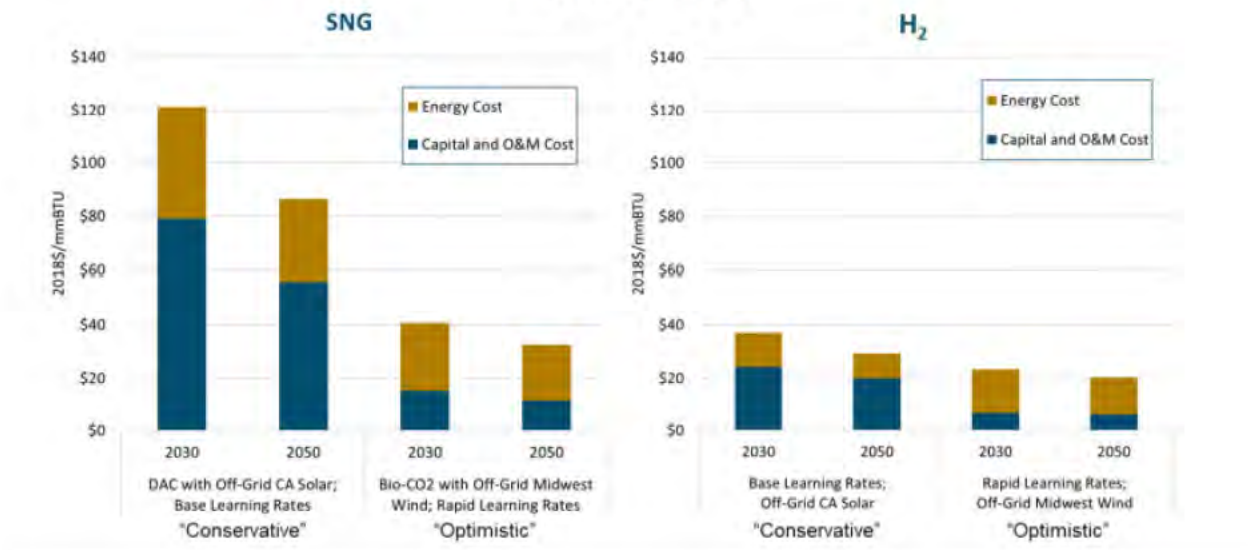
Figure 5: Power to Gas Commodity Costs for Production From a New Plant in 2030 or 2050
