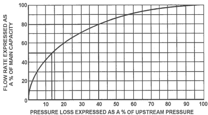
Figure 38. Relation between flow rate and pressure loss for a main operated at high pressure. 19
