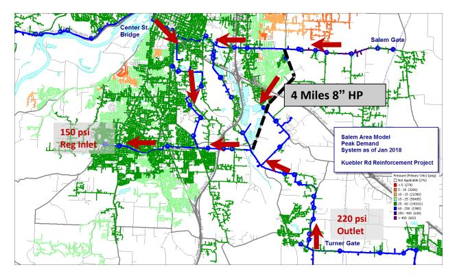
The Kuebler Road pipeline route was chosen as the preliminary pipeline design for the Kuebler Road Reinforcement Project.
