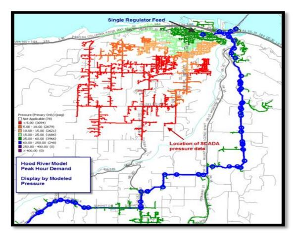
The location of the single SCADA point in this area is demonstrated above on the middle right; as the map demonstrates, there is only one SCADA point in this area.
