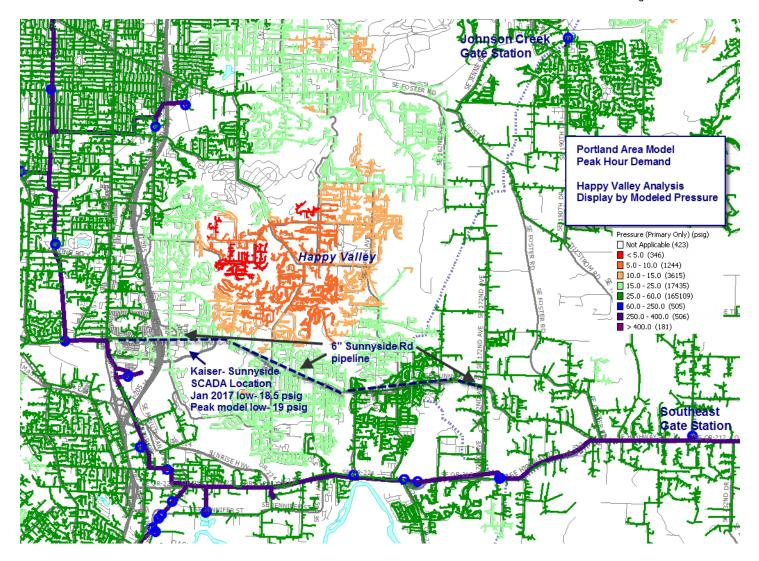
Modeled low pressures violates our system reinforcement criteria for lower pressure systems which specifies that 10 psig is the lowest acceptable pressure experienced or modeled in a distribution system. The10 psig threshold is driven by Excess Flow Valves which according to manufacturer specifications, are not designed to operate properly below that pressure. System reinforcement actions must be taken to assure safe and reliable service to firm customers in Happy Valley.
