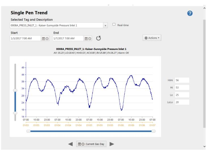
The mornings of January 5 & 6, 2017 saw low pressures of 20 psig and 18.5 psig respectively at the Kaiser location. These pressure reads by themselves do not violate any standards but indicate a very weak pipeline backbone that cannot properly support customer demands under peak conditions.
