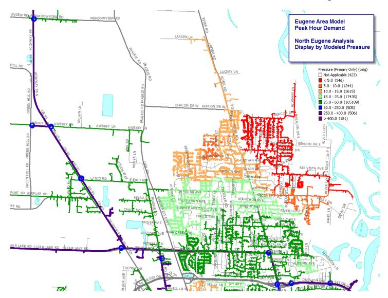
Modeled low pressures violate our system reinforcement criteria for lower pressure systems which specifies that 10 psig is the lowest acceptable pressure experienced or modeled in a distribution system. The10 psig threshold is determined by Excess Flow Valves which according to manufacturer specifications, are not designed to operate properly below that pressure. System reinforcement actions must be taken to assure safe and reliable service to firm customers in North Eugene.
