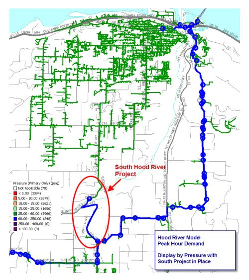
The southern project was selected as the preliminary pipeline design for the Hood River Reinforcement Project.
