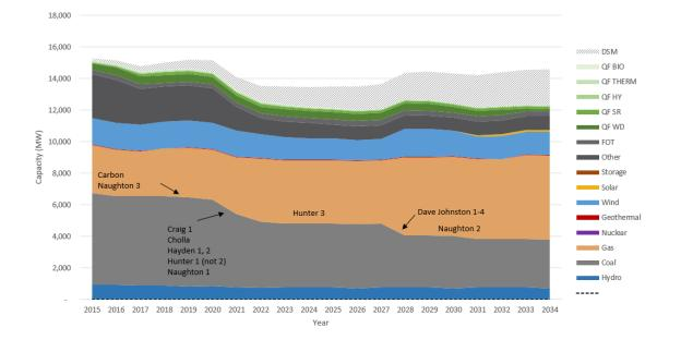
Figure 5. Generation capacity by year: Alternative IRP with 1) endogenous retirements, 2) mass-based CPP compliance (low CO<sub>2</sub> price), 3) adjusted decommissioning costs, 4) improved wind and solar capital cost assumptions, and 5) forced Dave Johnston 1-4 retirement in 2028
