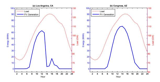
Figure 3. Hourly loads and dispatch of a fixed-axis PV plant located in Los Angeles, California, and Congress, Arizona, on July 20, 2005
