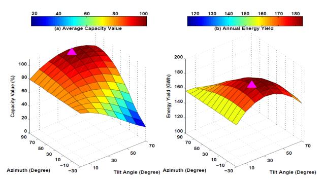
Figure 7. Average annual capacity value and energy yield of PV at Congress, Arizona, as a function of azimuth and tilt angles. Magenta triangles show the maximum.
