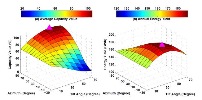
Figure 8. Average annual capacity value and energy yield of PV at Yucca Flat, Nevada, as a function of azimuth and tilt angles. Magenta triangles show the maximum.
