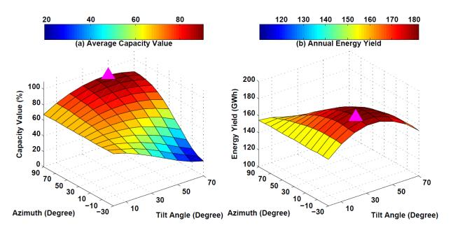
Figure 9. Average annual capacity value and energy yield of PV at Hanover, New Mexico, as a function of azimuth and tilt angles. Magenta triangles show the maximum.
