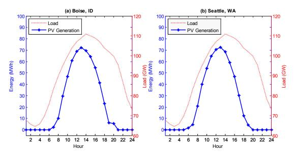
Figure 4. Hourly loads and dispatch of a fixed-axis PV plant located in Boise, Idaho, and Seattle, Washington, on July 10, 2002
