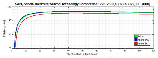
Figure 1. Inverter efficiency curve<sup>8</sup>
