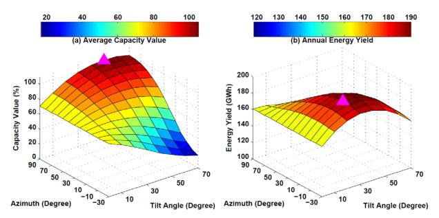
Figure 6. Average annual capacity value and energy yield of PV at Bartsow, California, as a function of azimuth and tilt angles. Magenta triangles show the maximum.
