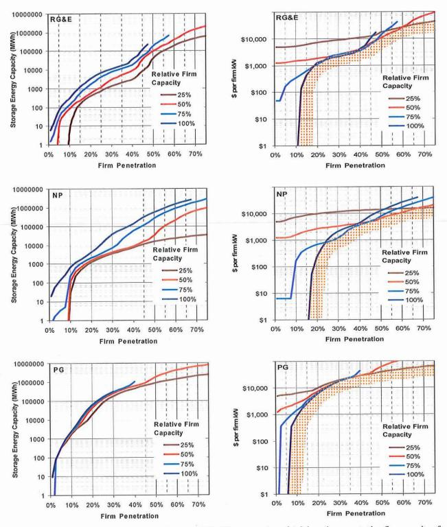
Figure 3: Energy Storage Requirements (left) and cost (right) necessary to maintaining a low-penetration firm capacity of 75% as a function of firm PV penetration. Costs are reported in terms of \$ per firm kW delivered.
