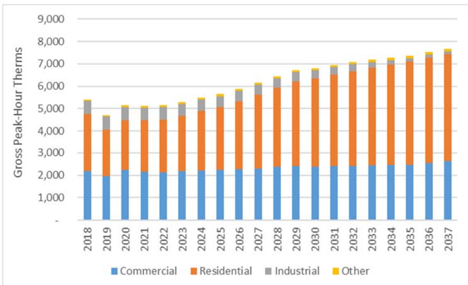
Figure E.10: NW Natural’s Annual Peak Hour Savings Projection for Oregon by Sector
