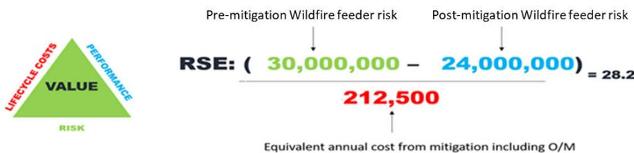
In this hypothetical example, undergrounding the line (Example 1) would yield a higher RSE value—risk reduction per dollar of investment—than Example 2 (reconductoring the line and installing fire-safe fuses): an RSE value of 90:1 vs. 28:1.
