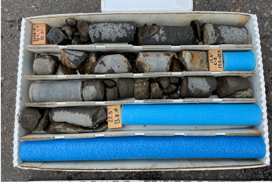
BORING B-1, 12.5 FEET TO 22.5 FEET
