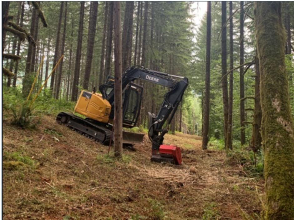
**Figure 23. SlashBuster Clearing Right of Way**
