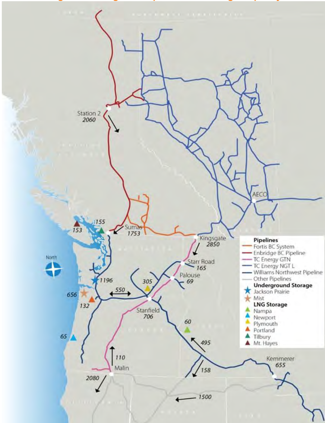
Figure 4.7: Regional Pipeline and Storage Capacity
