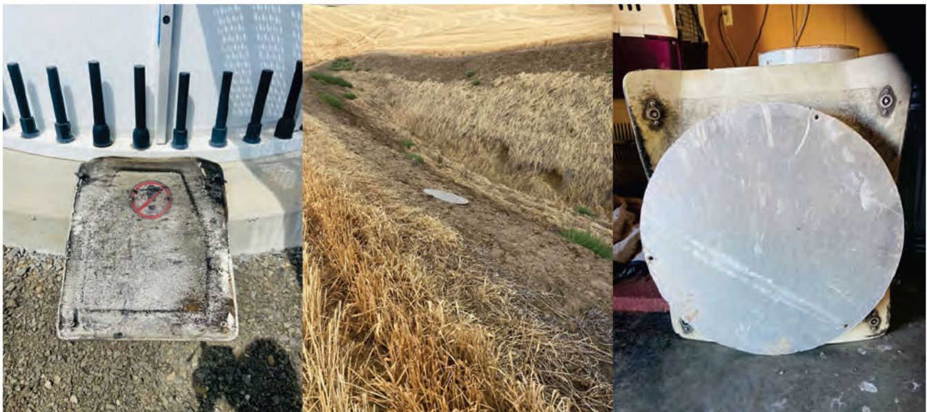
Landowners say they find hatch doors (left) from the Vestas turbines at Biglow Canyon and metal disks (center) from the Siemens turbines that break off and fall into their fields from a height of about 265 feet. State regulators say even small objects falling from that height can reach speeds of nearly 90 mph and could endanger anyone below. (Courtesy Kathryn McCullough)
