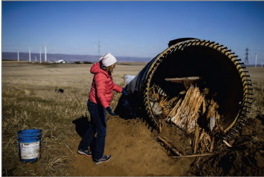
Kathryn McCullough, a Sherman County landowner, examines the blade that was thrown from a turbine at PGE's Biglow Canyon wind farm on Feb. 1. Her husband, Kevin McCullough, farms wheat under about half the wind farm's 217 turbines, including the one that threw the blade. Thirteen of the wind farm's turbines are on their land.
