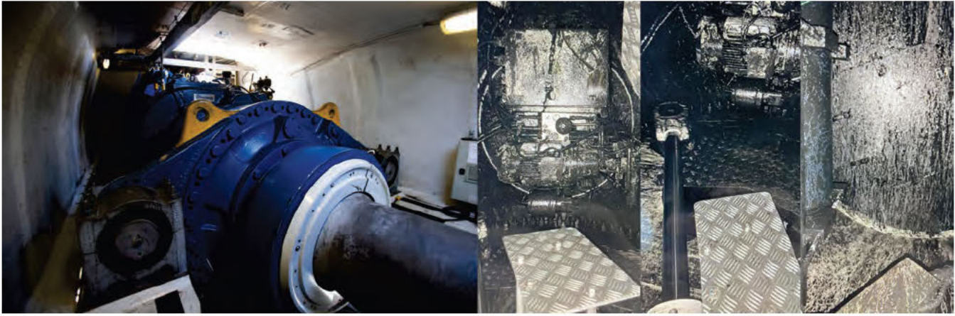
Portland General Electric provided a look inside the spotless nacelle of a Vestas turbines (left) at Biglow Canyon wind farm during a tour in late June. Kathryn McCullough sent the pictures at right to U.S. Sen. Ron Wyden, which she said shows the oil-coated nacelle of a Vestas turbine this spring at Biglow Canyon. (Photos courtesy PGE, left, and Courtesy Kathryn McCullough, right)
