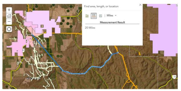
Option A is an alternate route that leaves the proposed route at MP 19.3 and continues its South East trajectory to the point on Spur Loop Road that intersect the Wheat Ridge Renewable Energy Facility East. It parallels the Wheat Ridge corridor south of Gleason Butte, departs the corridor at Ayers Canyon and reconnects with the proposed route at MP 36.
