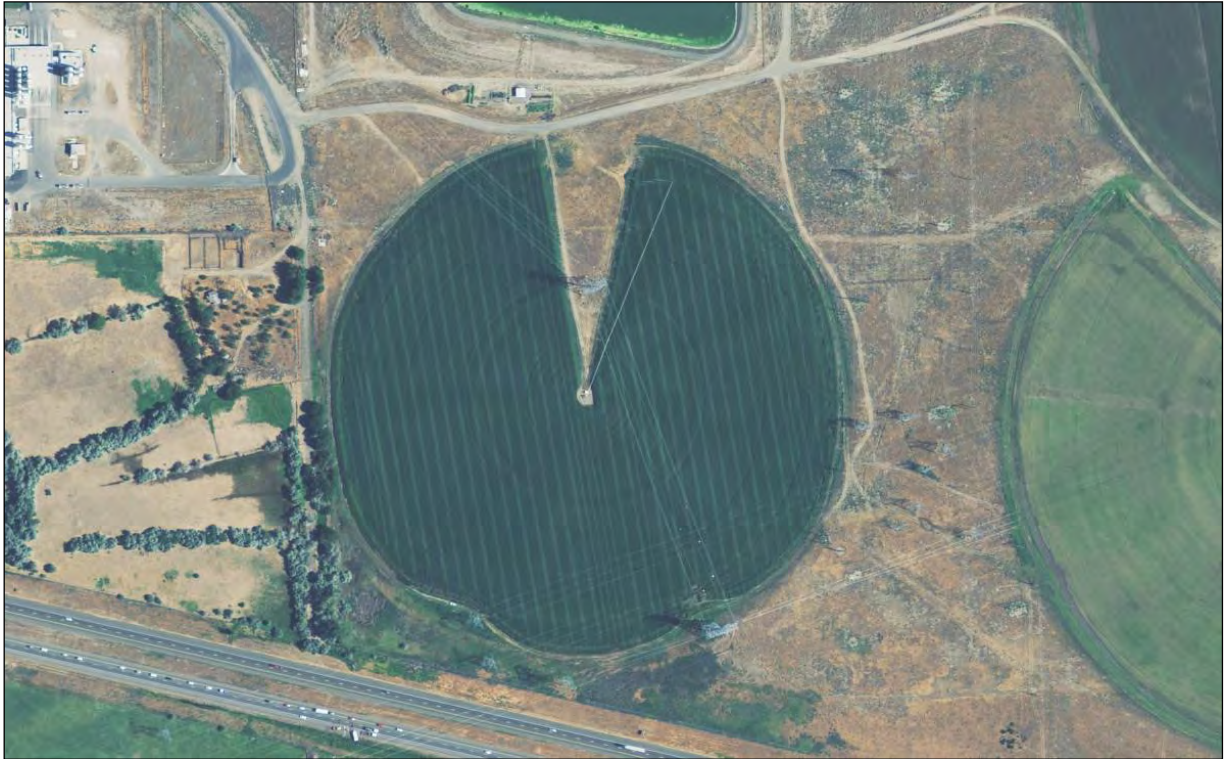
Figure 5-2. Aerial Photograph Showing Reduced Farmable Acreage within a Center-Pivot-Irrigated Parcel Resulting from the Placement of a Transmission Line Tower (approximately 2 acres of this 40-acre field are lost to production because of the presence of a transmission line tower)
