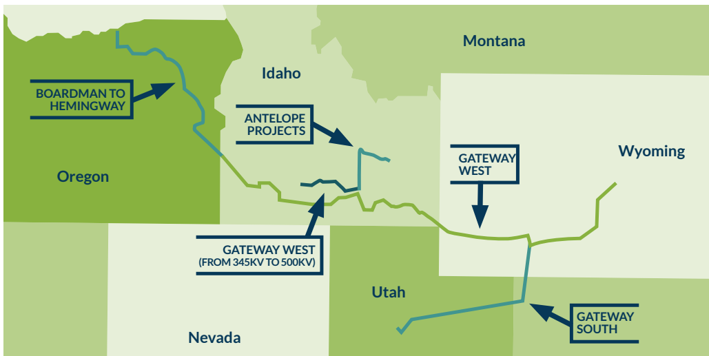
FIGURE 14 These projects comprise NTTG’s final RTP.
