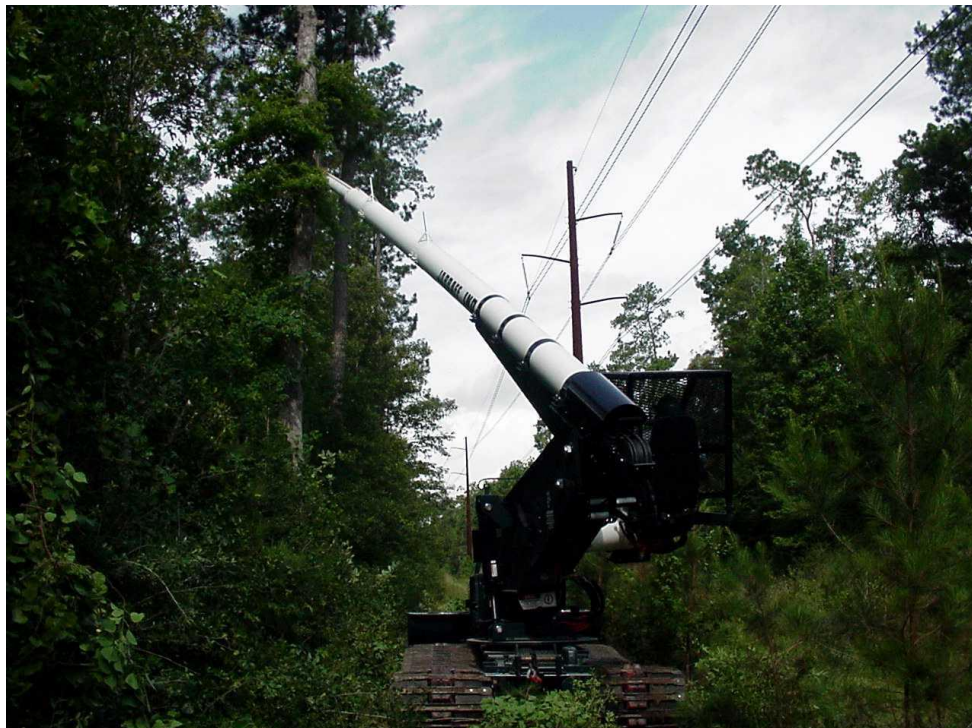
Figure 2.5. Jarraff mechanical "trimmer" that may improve productivity in remote areas.
