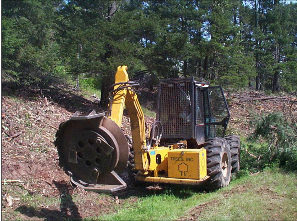
Figure 2.5. Jarraff mechanical "trimmer" that may improve productivity in remote areas.
