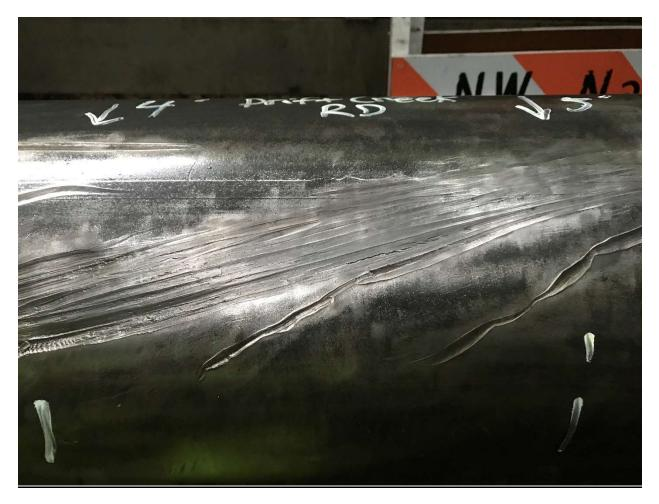
Figure #3 Metal loss caused by cable dragging along pipe
