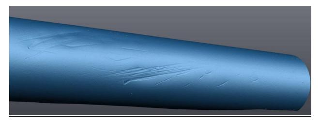
Figure #2 Scanned image of damage caused by cable
