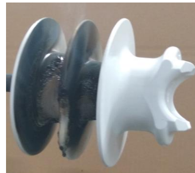
Image 2: Flame self-extinguished after heat source is removed.
