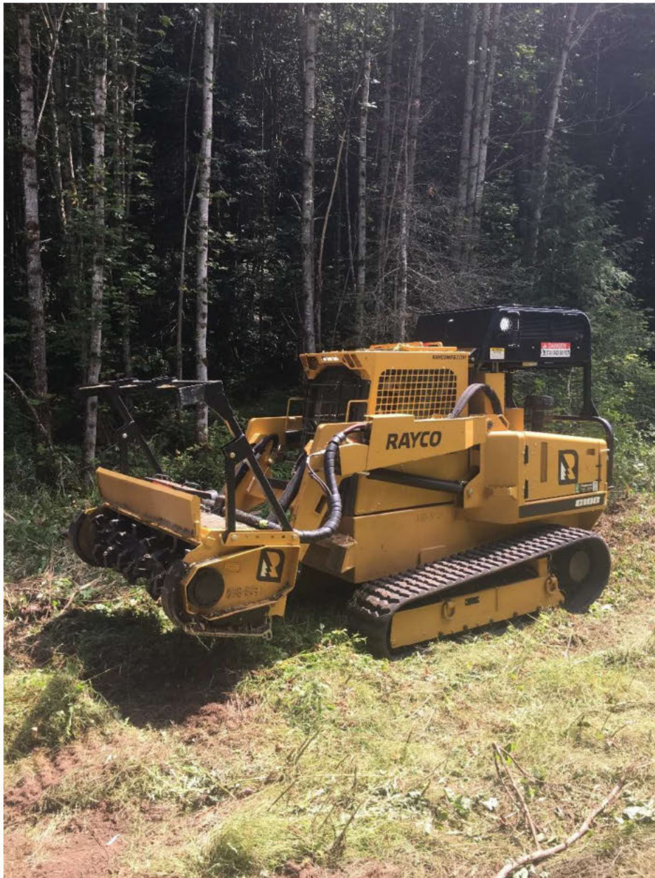
FIGURE 6: SLASHBUSTER HEAVY-DUTY FORESTRY MOWER
