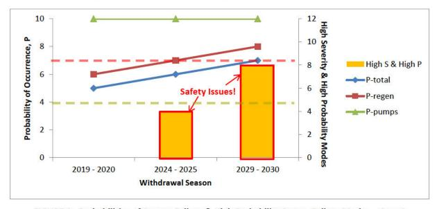
FIGURE 1: Probabilities of System Failure & High Probability Severe Failure Modes – Case 1
