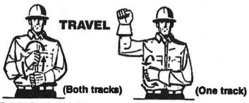
Both fists in front of body, making a circular motion about each other, indicating direction of travel; forward or backward,
