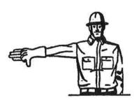
With arm extended, thumb down, flex fingers in and out as long as load
