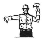
LOWER THE BOOM AND RAISE THE LOAD Arm extended, fingers closed, thumb down, other arm vertical, forefinger upward and rotate hand.
