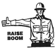
Arm extended, fingers closed, thumb pointing upward.
