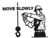
Use one hand to give any motion signal and place other hand motionless in front of hand giving the motion signal (Hoist slowly shown as example.)
