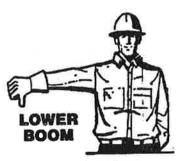
Arm extended, fingers closed, thumb pointing downward.
