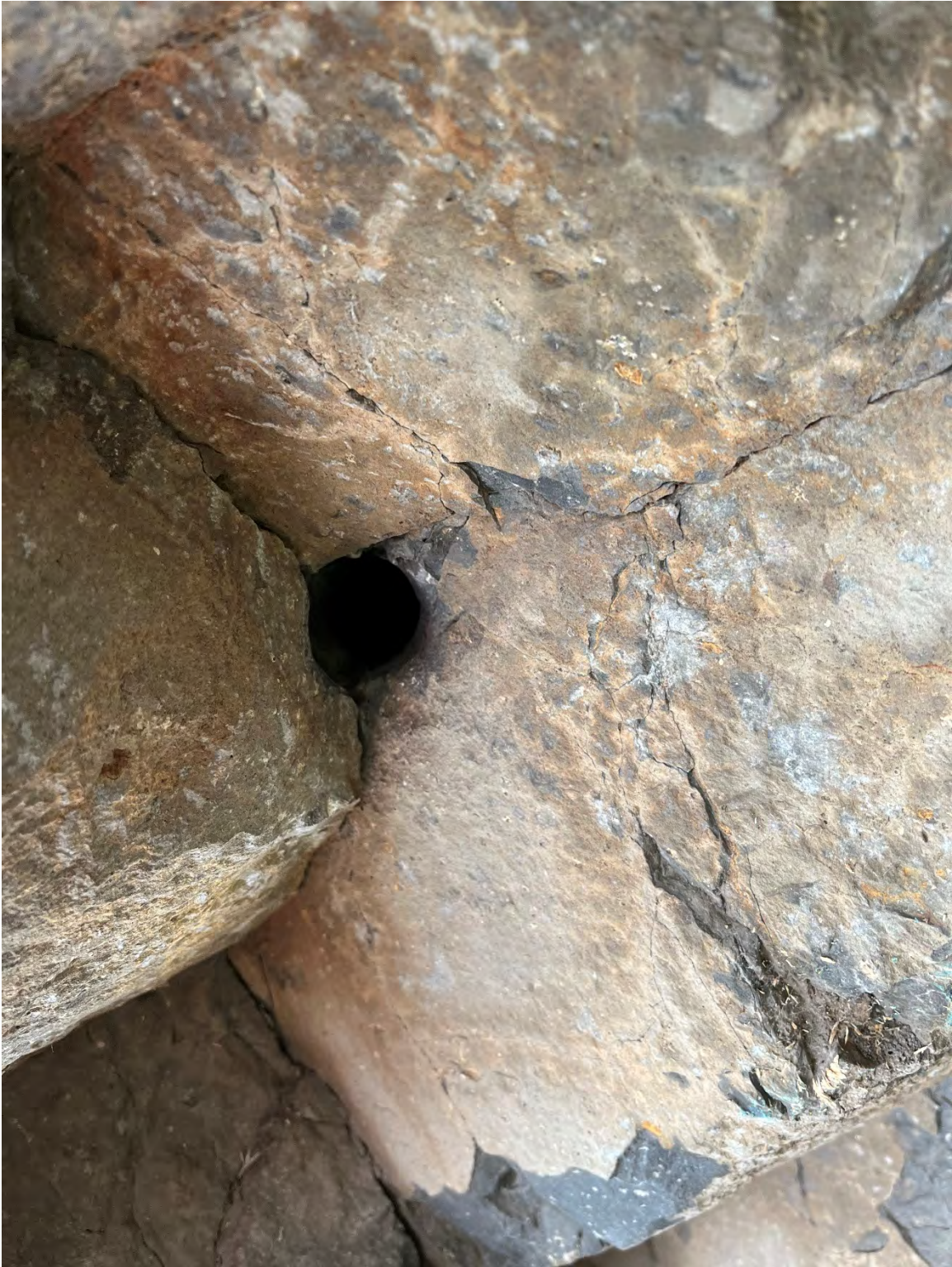
Photograph 8: Evidence of Former Dynamite Usage
