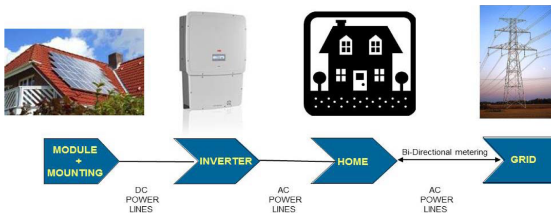
FIGURE 7-2: Distributed solar PV system
