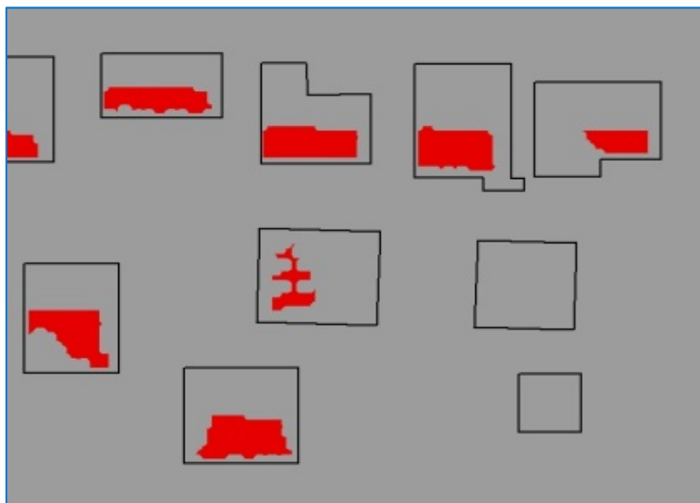
Figure B-4 Tilted Roof Planes Meeting Solar Cutoff and Setback Requirements (red areas indicate areas meeting cutoff and setback requirements)
