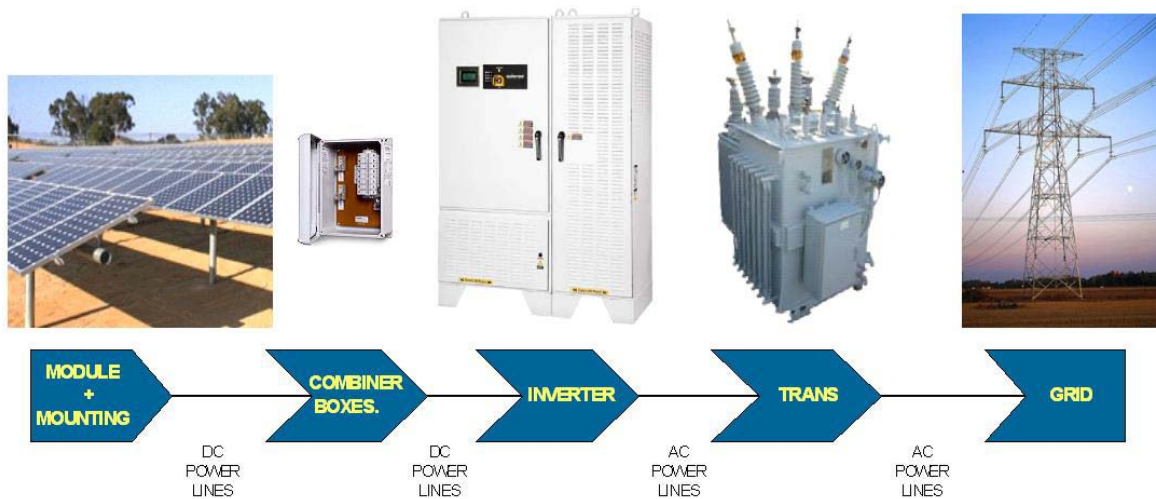
Figure 3-2 Example Components for Utility-Scale Solar PV System
