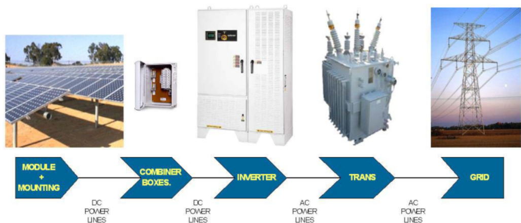
FIGURE 7-9: Centralized solar PV system
