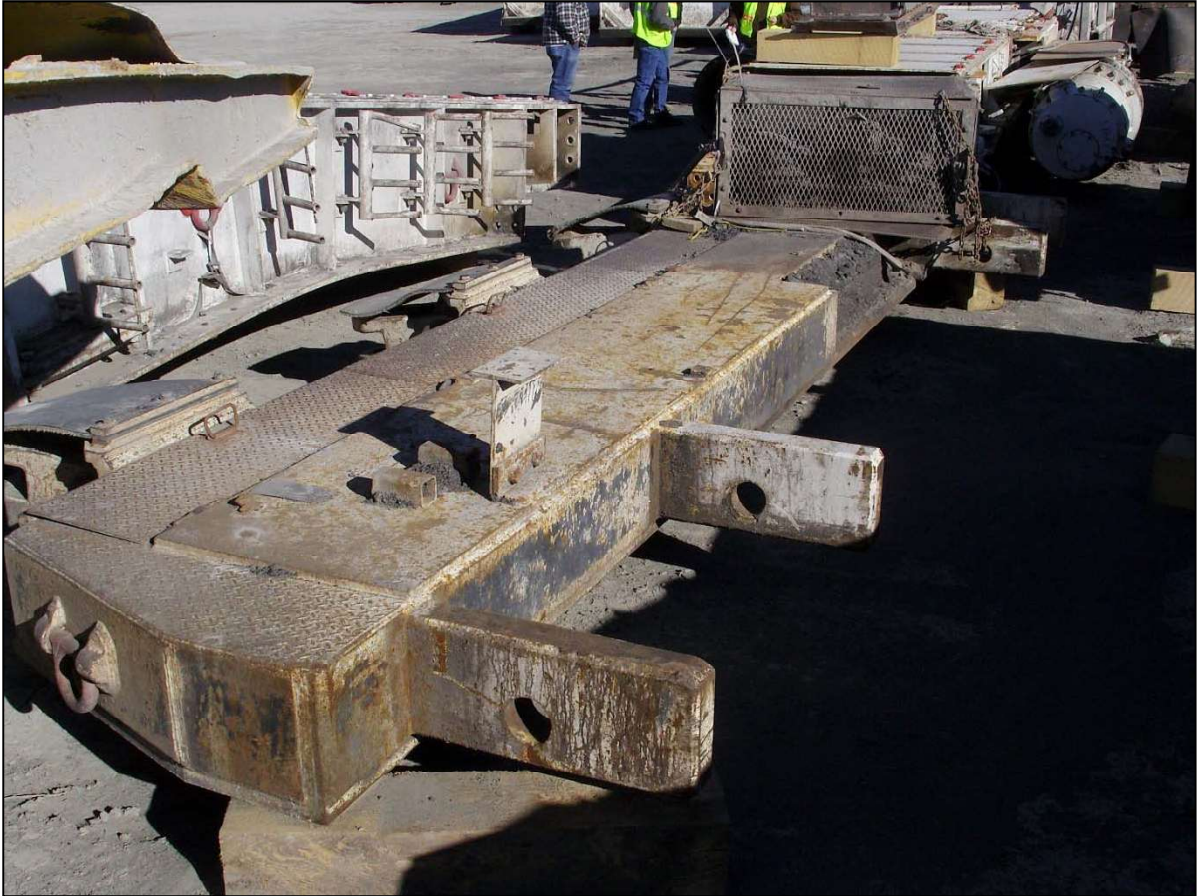
Headgate Drive Platform, 22-185
