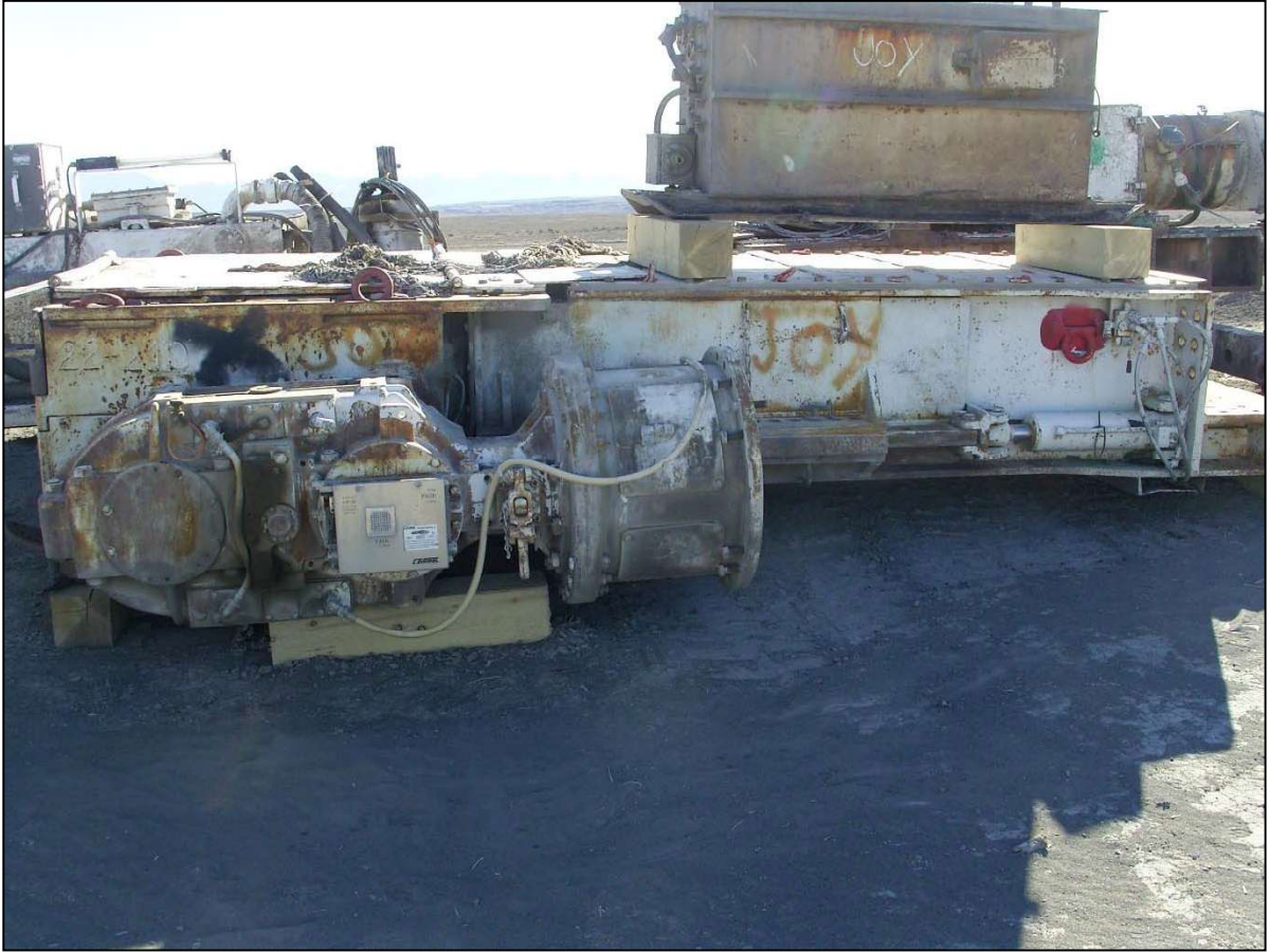
Stagloader Drive Assembly, 22-210
