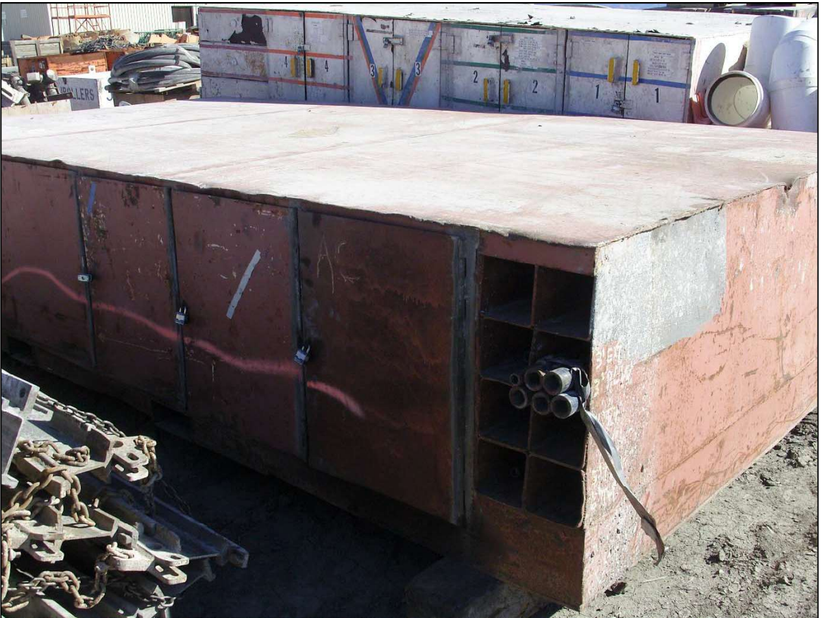
Support Skid with Tool Boxes
