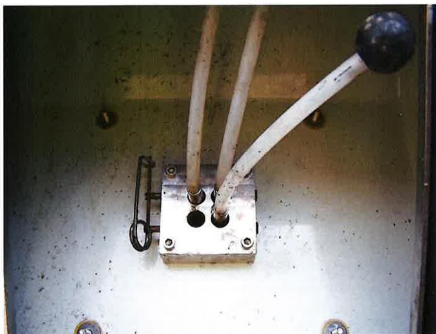
Figure 1.6 ECA Rod Assembly Inside the Source Cartridge Door
