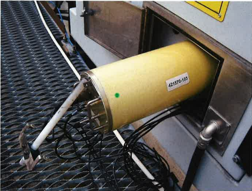
Figure 1.8 ECA Detector Section – Partially Removed
