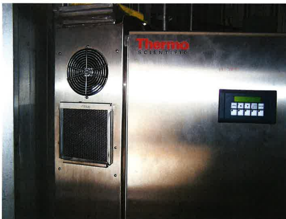
Figure 1.11 ECA Analyzer Electronics Module with Exhaust Fan and Filtered Inlet
