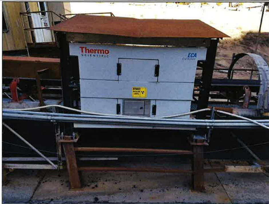
Thermo Scientific Elemental CrossBelt Analyzer™ (ECA) located at Deer Creek Mine Emery County, Utah
