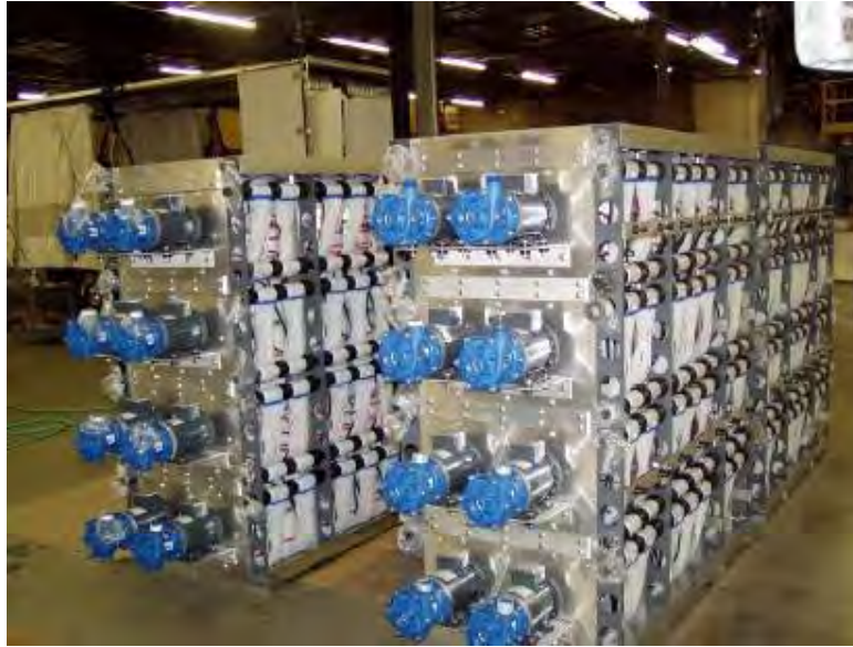
Figure 15 - ZnBr Cell Stacks
