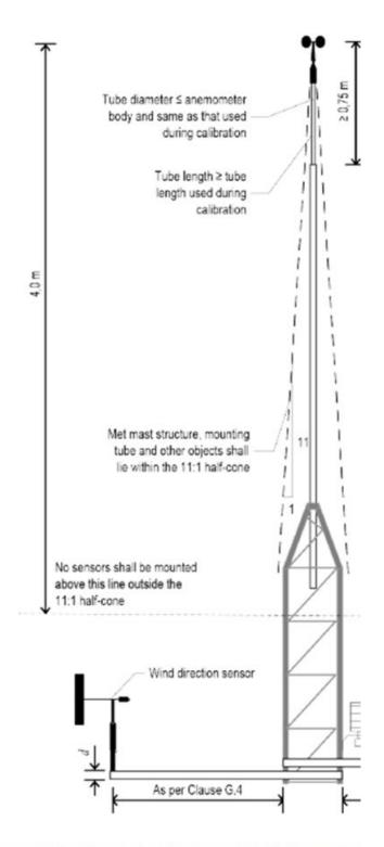
Figure G.1 - Example of a top-mounted anemor
