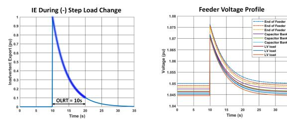
**Figure 7.** Case 6 Urban Feeder: Coincident Inadvertent Export Curve (Left) and Time Series RMS Maximum Voltage Profiles (Right)
