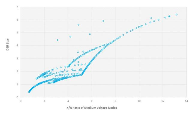
Figure XI. 4. Non-Exporting DER Size at Each Node Based on the PCC Short CircuitMVA/DERMVA = 25
