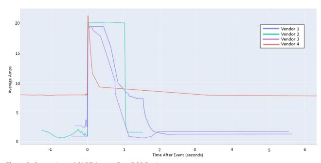
**Figure 2.** Comparison of OLRT Among Four PCS Devices **Note:** The four devices took an average of 1.173 seconds to return to steady state (within 5% of prior current) at an average current of 11.757 amps.
