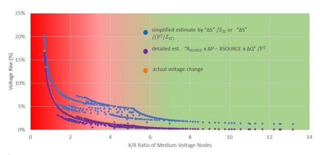
Figure XI. 3. Voltage Change Calculated Along a Feeder for a 2 MW Change in Export at Each PCC
