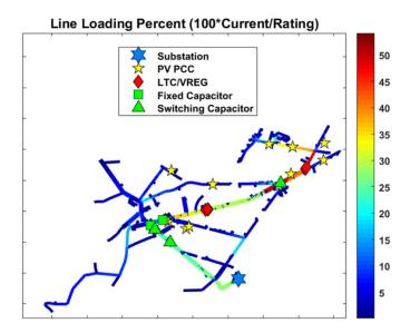
**Figure XI. 18.** Rural Feeder: Line Loading With Maximum Solar PV Output Under Minimum Load Conditions **Note:** The gradient bar on the right side of the figure shows the percentage of the line's current ratings.
