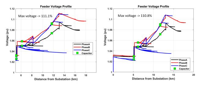
**Figure 10.** Rural Feeder: Overvoltage Violations at 30 Seconds OLRT (Case 5) at Right, and 10 Seconds OLRT (Case 6) at Left
