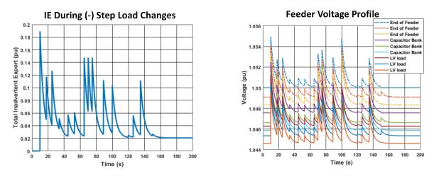
**Figure 6.** Case 8 Urban Feeder: Inadvertent Export Profile (Left) and Time Series RMS Maximum Voltage Profiles During the Same Time Period (Right)
