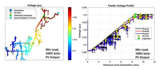
Figure 3. Case 1 Urban Feeder: Voltage-Level Map (Left) and Coincident RMS Maximum Voltages Along the Feeder (Right)
