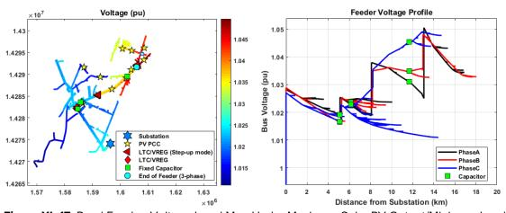
**Figure XI. 17.** Rural Feeder: Voltage Level Map Under Maximum Solar PV Output/Minimum Load (Left) and RMS Maximum Voltages Along the Feeder (Right)
