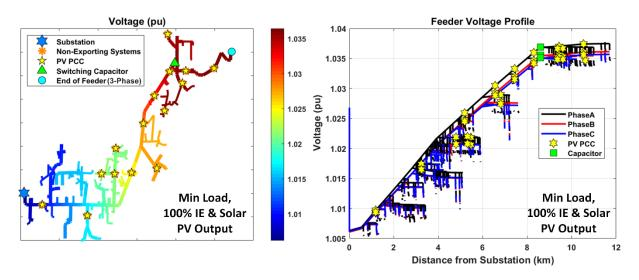
**Figure 4.** Case 5 Urban Feeder: Voltage-Level Map (Left) and Coincident RMS Maximum Voltages Along the Feeder
