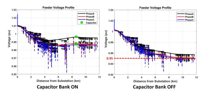
Figure XI. 7. Voltages Along the Urban Feeder With Capacitor Bank On (Left) and Off (Right)
