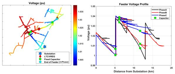
Figure XI. 16. Rural Feeder Voltage Profile
