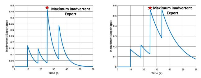
**Figure XI. 19.** Rural Feeder: "Rapid Fire" Inadvertent Export Profile With 10s OLRT (Left) and 30s OLRT (Right)
