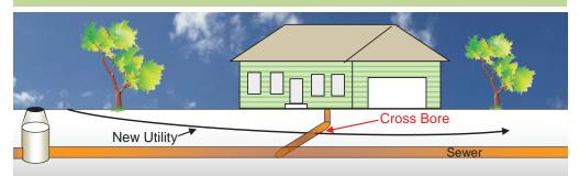
Be alert when unblocking an underground sewer line. A cross bore could exist and cause a natural gas emergency. In areas where trenchless technology has been used to install underground utility lines, there is a possibility that our gas pipeline may cross through a sewer pipe, resulting in a cross bore.
