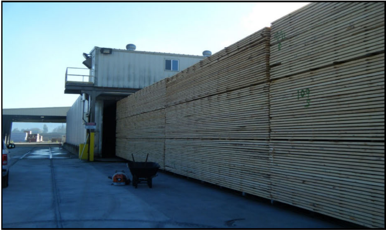
Kiln-12 – Stacked lumber from the sawmill ready to go into the kiln for drying.
