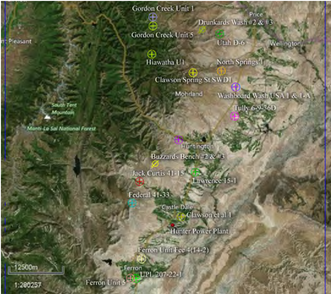
Figure 30. Proposed well locations for the CarbonSAFE Rocky Mountain CCS project, Buzzards Bench #2 & #3 and Drunkards Wash #2 & #3 along with 17 other plugged and abandoned wells that could be used for a regional CCS site. The blue rectangle is the model boundary. The CO 2 injection wells are indicated with white labels.
