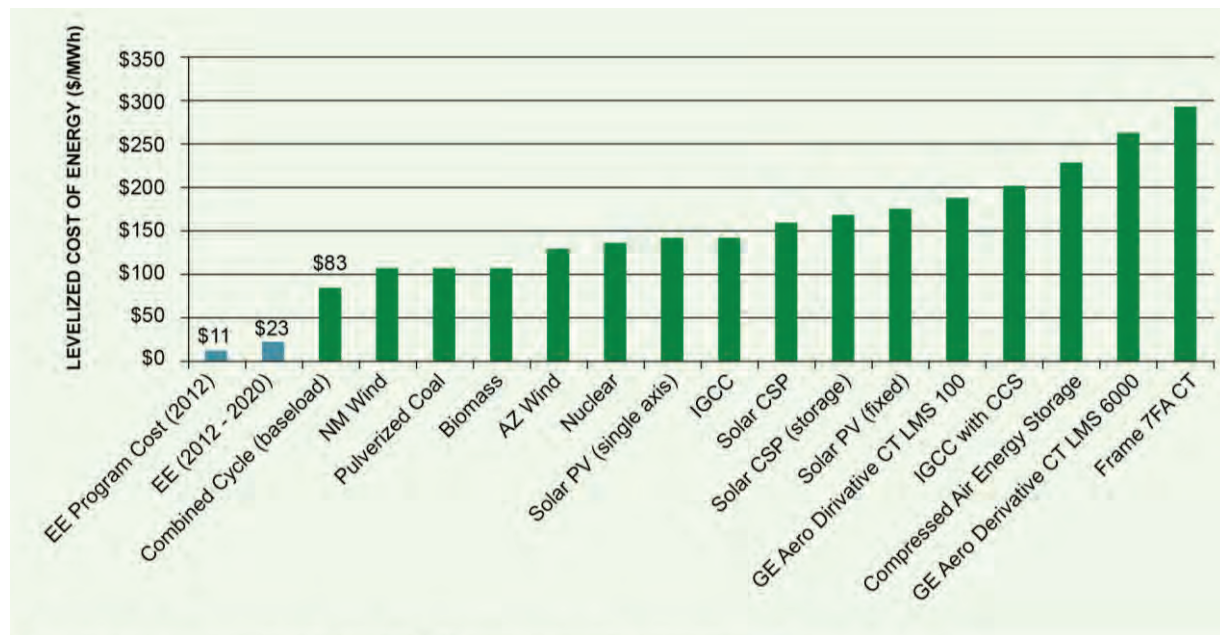
Conventional resource costs include fuel, capital, O&M, transmission, and interconnection costs. Renewable resource costs include generation, delivery, backup capacity, and system integration costs. Data Source: Tucson Electric Power 2012 IRP, 2012 DSM Report, and 10/31/2012 TEP Rate Case Technical Conference
