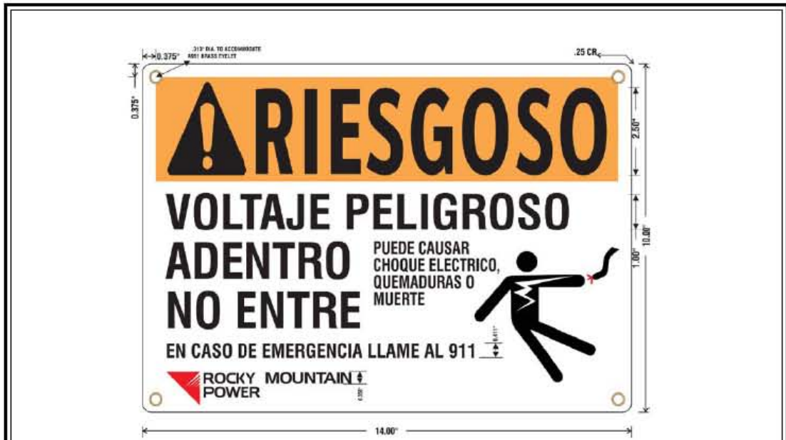
Figure 4—Spanish High-Voltage Warning Sign for Rocky Mountain Power (SI# 7999854)
