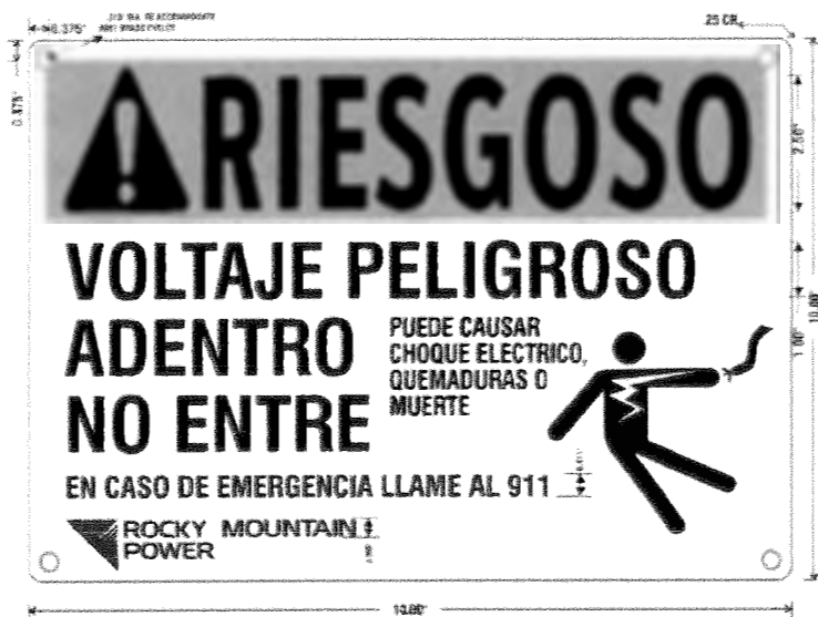
Figure 4—Spanish High-Voltage Warning Sign for Rocky Mountain Power (SI# 7999854)
