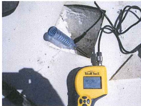
Probes inserted at facer of polyiso insulation layer.
