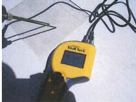
Probes inserted into core of cover board.
